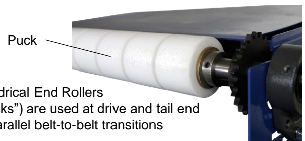
90-deg. Square-Turn with 2.5" Pucks with Underslung Drive, in Stainless Steel Design
